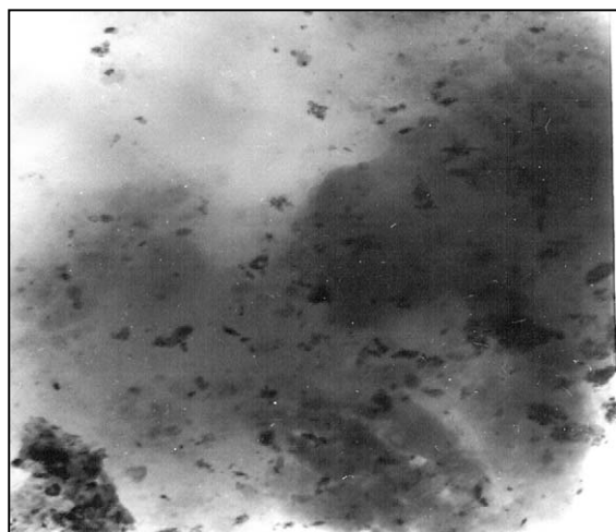
Figure 4. SEM micrograph of the hydrogen activated 4% Pd/PVP catalyst (magnification \times 500 ).
